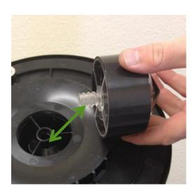
There is a screw to the base as circled below; this needs to be removed to release the foams.
