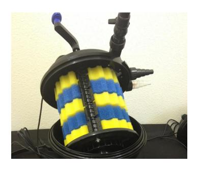
20000 Model- There are three layers of yellow foam and two layers of blue.
